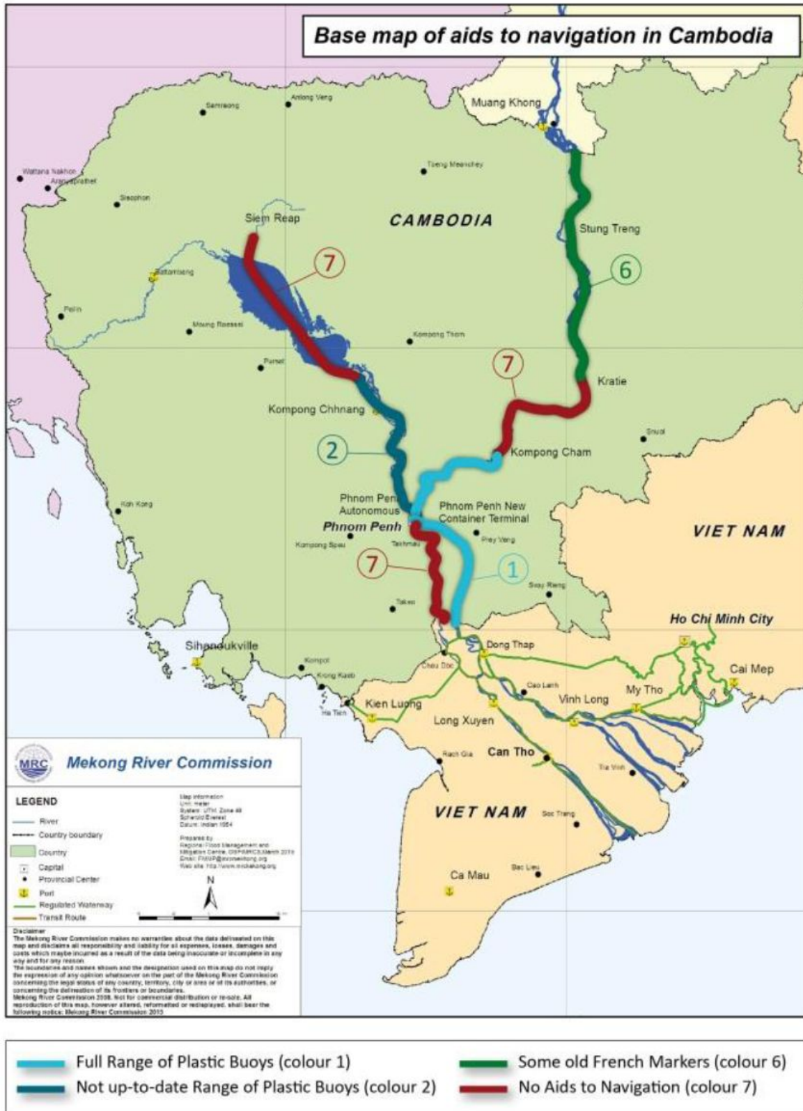
Figure 2. Existing navigation aids in Cambodian waterways, from MRC (2015)
