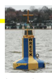
An Emergency wreck buoy is used to warn of a new wreck which has not yet been listed in maritime documents. The buoy is expected to be deployed for the first 24-72 hours after the wreck occurs. After that time more permanent buoyage (such as isolated danger marks or cardinal marks) should be deployed and charts updated.
