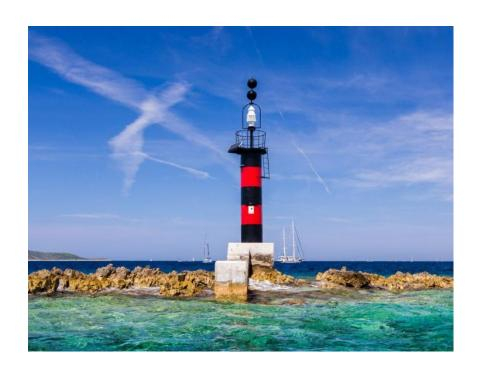
An Isolated Danger Mark, as defined by the International Association of Lighthouse Authorities, is a sea mark used in maritime pilotage to indicate a hazard to shipping such as a partially submerged rock.
